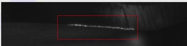
Image 6: Subimage of cutter number 2, the damage is clearly visible and detectable by vision, damage size width: 4.9  $\mu\text{m}$ ; length: x: ~1100  $\mu\text{m}$
