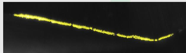
Image 10: result of the edge detection algorithm detecting the edges of the damage.
