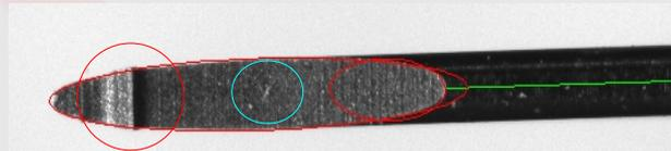
Image 9: Dynamic contrast measurements detect the irregularities in the cut surface.
