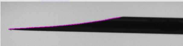
Image 1: Side view of a well produced needle, in purple the detected contour points of the cut surface.
