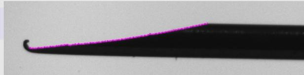
Image 3: needle with bent tip, the fit is executed over the purple dots on the 'cut surface'.
