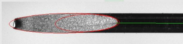
Image 11: The two ellipse fits and the middle line of the shaft.
