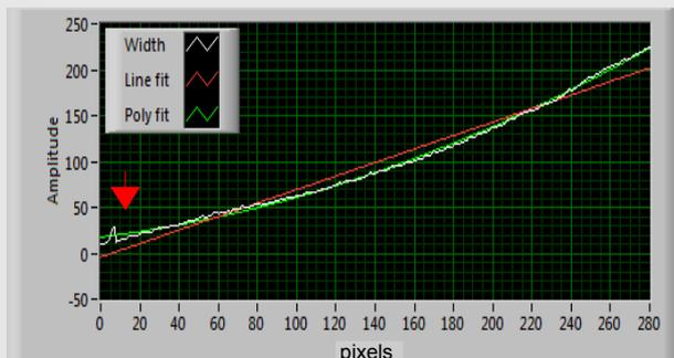
Image 2: Width of the needle (white). Linear fit in red and a parabolic fit in green.
