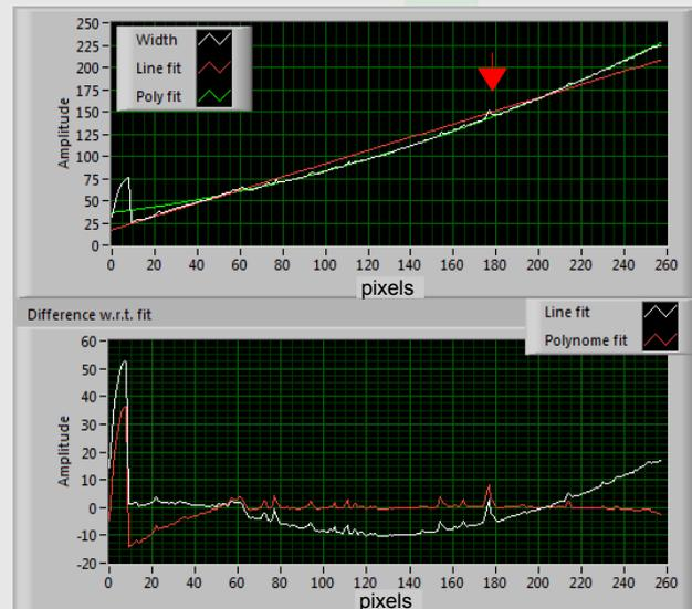
Image 4: Above the measured points are displayed in white above. The red line indicated the linear fit and the green line indicates a polynomial fit. Below displays the difference between measured points and both fits.
