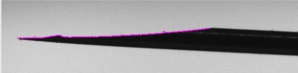
Image 5: Poorly produced needle, 'lump' in cut surface.
